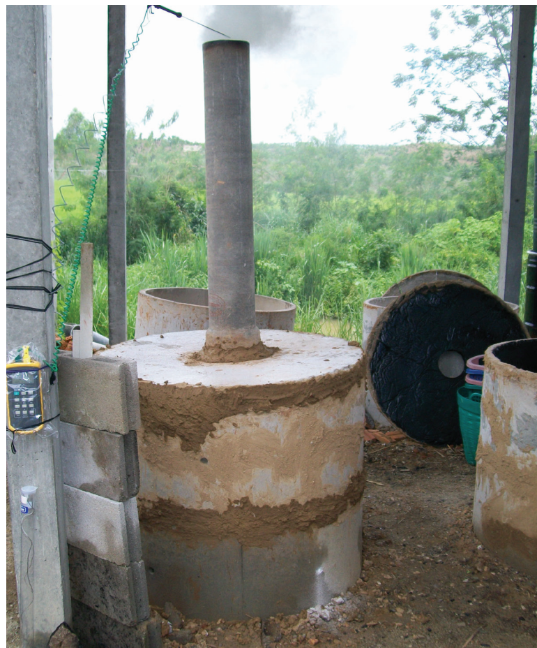
Controlled Temperature Biochar Retort for Slow Pyrolysis Process
