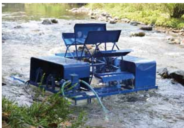
Figure 2 Water turbine driven the piston pump (Chula-Pidthong 6)
