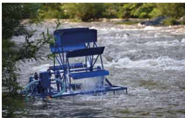
Figure 1 Water turbine Chula-Pidthong 8 (the latest development model). Experimental turbine installed at The Kaeng Krachan National Park Ranger 10 (Huai Mae Saliang) Photographed by: Boonpeng, March 2017
