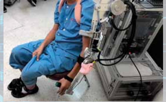
Figure 3 Installing a robotic arm to the arm requiring assistance Source: Sangveraphunsiri (2014)
