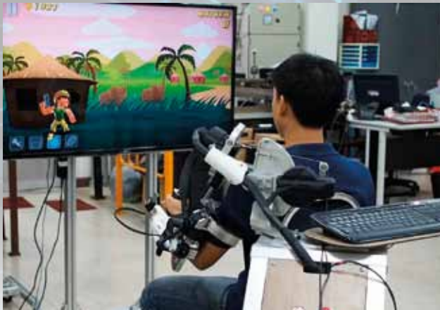
Figure 8 Test robots arm CUREs and training game Source: Sangveraphunsiri (2017)
