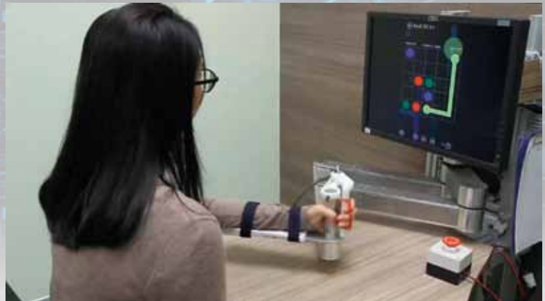
Figure 6 The end-effector type is used for rehabilitation in stroke patient Source: Sangveraphunsiri (2017)
