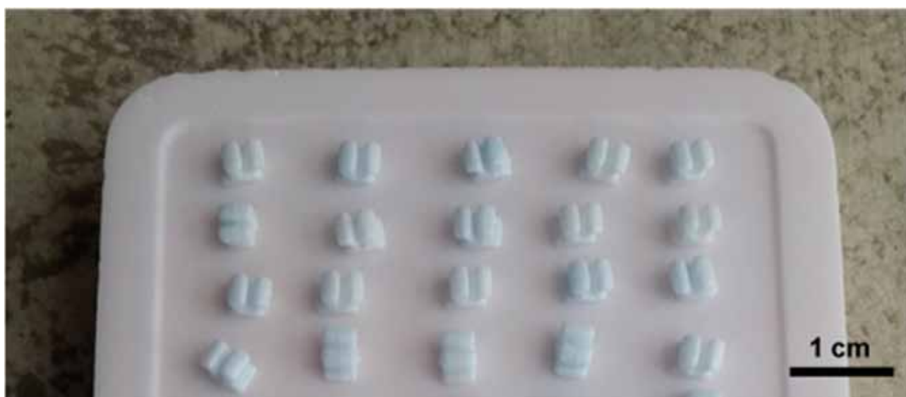
Figure 5 Ceramic brackets produced in the study Photographed by: Wasanapiarnpong, 17 July 2017
