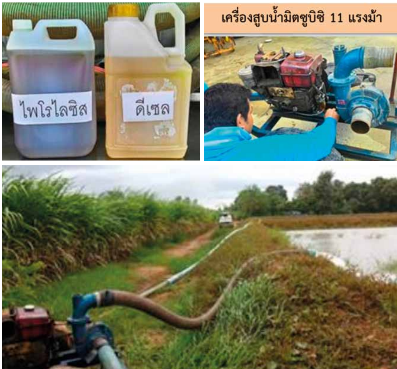
Figure 6 Using pyrolysis oil for agricultural engines Source: Energy Research Institute (2014)
