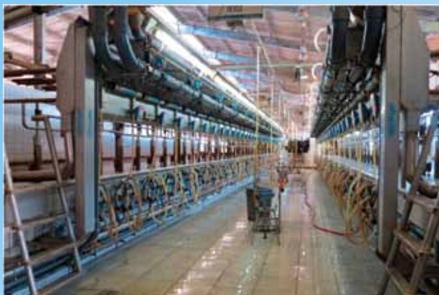
Figure 9 Pipeline milking system of a large dairy farm in Vietnam Source: Ajariyakhajorn (2016)
