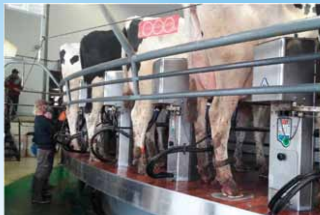
Figure 10 Rotary milking system of a large dairy farm (2,000 cows) in Wisconsin, USA Source: Ajariyakhajorn (2016)
